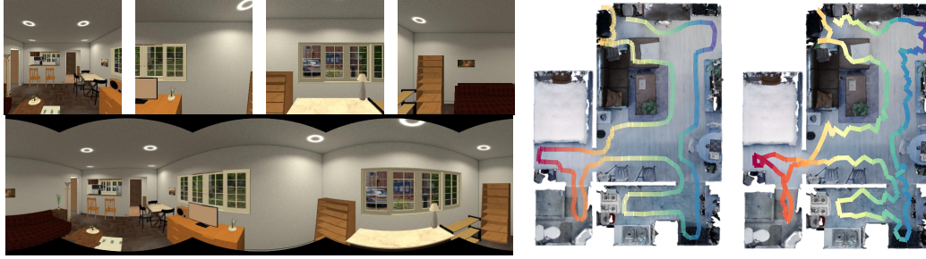
Figure 4: An example of the iGibson environment; (left) the quadruple-view at the location of observer and the constructed panorama image; (middle) a ground truth trajectory; (right) prediction
