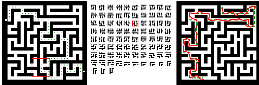
Figure 3: Synthetic maze environment of size 24 \times 24 pixels; (left) An example of a path and the sampling window; (middle) extracted patches for the shown path; (right) an example of the ground truth (in green) and the predicted (in red) trajectories
